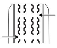
the same height as these "wear bars", the tire is worn out and must be replaced.
